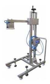
The pusher unit (DPP), as provided with wheels, can be integrated to the production line and it's managed from a software. Its function is to push down the top layer of cakes (cover). This operation is useful to make uniform the height of the cakes
